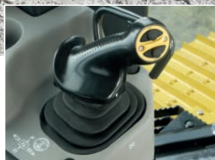
PCCS (Palm Command Control System)
